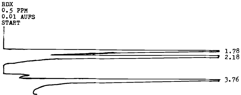
FIG. 2—Ten-microlitre injection of RDX standard solution (0.5 ppm).
